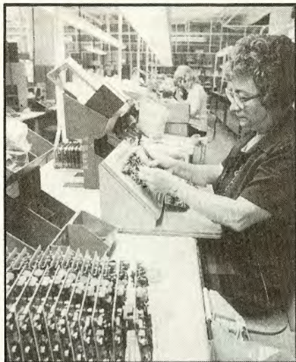
Circuit boards assembled by computer-controlled sequence.
