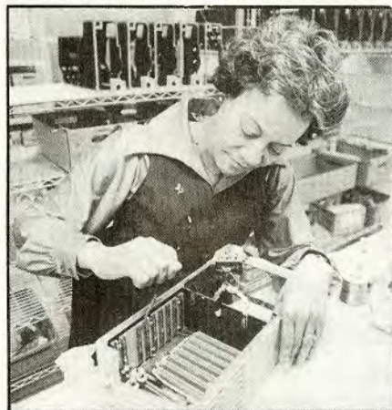
Assembled circuit boards are installed in TK-76 body frame.
